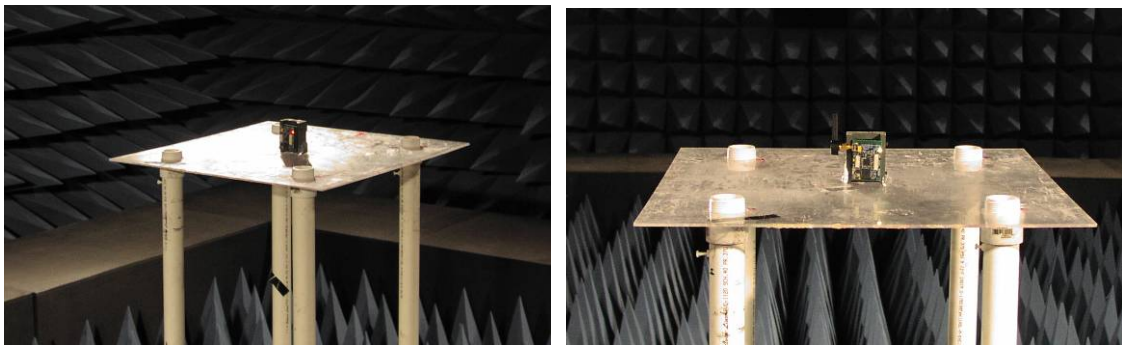
Figure 6.52 Onboard and external antenna set-up in anechoic chamber.
