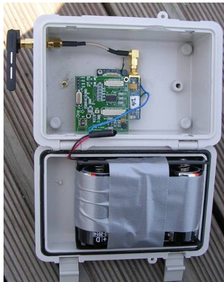
Figure 7.90 Sensor in enclosure with batteries and antenna for Jindo Bridge deployment.
