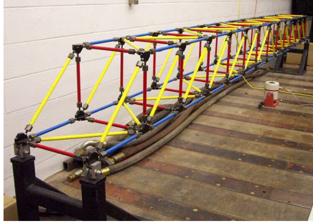
Figure 2.4 Three-dimensional truss model.
