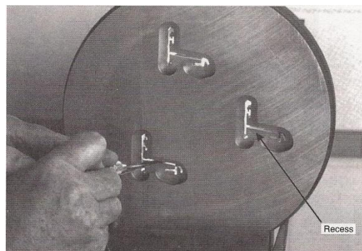
Figure 5.6 Example of a Recessed Solid Die [22].
