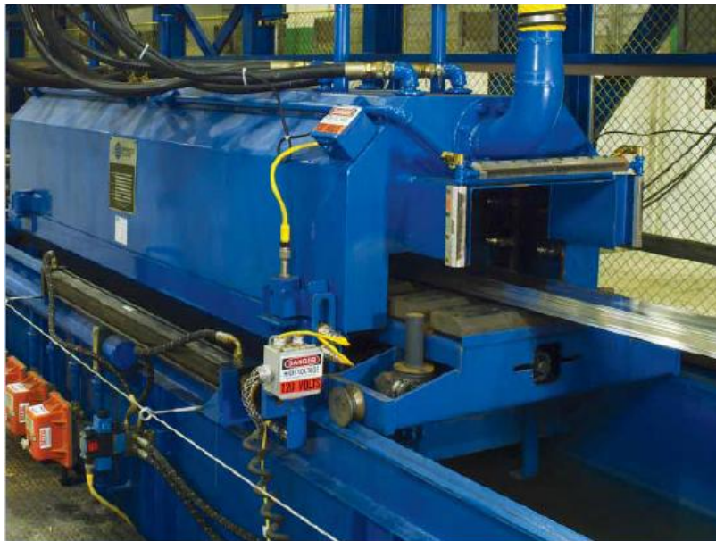
Figure 3.3 High-Pressure Spray Quench, from Granco Clark [28].
