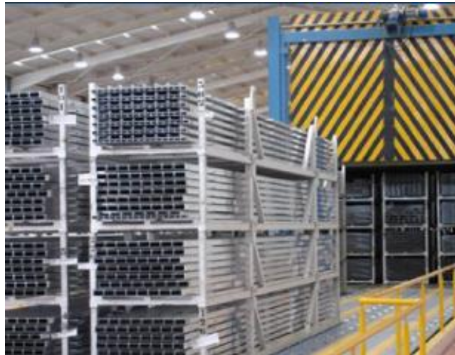
Figure 3.6 Racked extrusions going into the Aging Oven, from GiA CLECIM Press [32].
