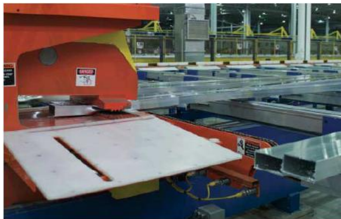
Figure 3.4 Granco Clark's Controlled Vertical Crush Stretcher (CVCS) in operation [29].
