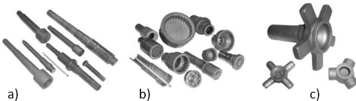
Figure 1.2 Parts made by (a) forward extrusion, (b) backward extrusion, and (c) lateral extrusion [6].
