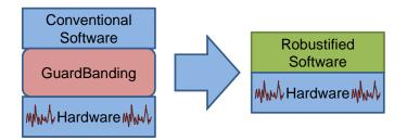
Figure 1.1: The traditional approach to dealing with hardware uncertainties is through guardbanding. We allow hardware errors to be exposed to software which is robustified to tolerate these errors.
