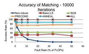
Figure 6.5: The effect of enhancements to gradient descent on the success rate of *bipartite graph matching*
