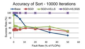
Figure 6.1: Success rate for different implementations of *sorting* as a function of fault rate
