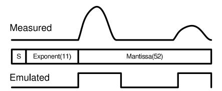
Figure 5.1: Measured distribution of error magnitudes for floating point data versus the distribution used for emulating the behavior.
