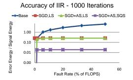
Figure 6.3: Error-to-signal ratio for different implementations of *IIR* as a function of fault rate (lower is better)
