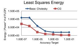
Figure 6.6: Accuracy for a CG-based implementation of *least squares* (10 iterations)
