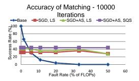
Figure 6.4: Success rate for different implementations of *bipartite graph matching* as a function of fault rate
