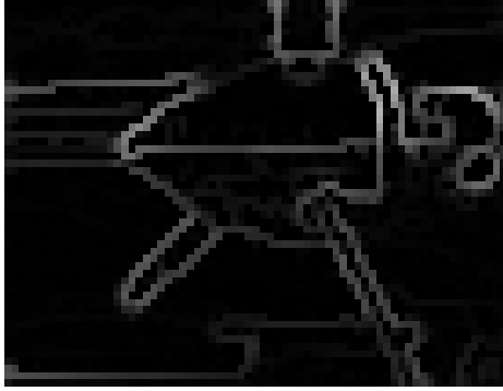
(a) The output of the new ramp detection method on the image in Figure 2.5(a). Compare this to the output of the ramp transform in Figure 2.5(b).
