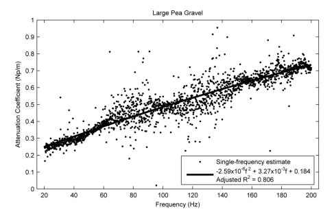
**Fig. 3.** Attenuation coefficient for large sifted pea gravel. Each dot is a separate determination of the attenuation coefficient by the LMSE process for a distinct frequency.
