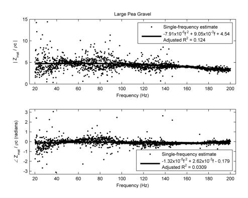
**Fig. 5.** Characteristic impedance for large sifted pea gravel normalized by ρc for air.
