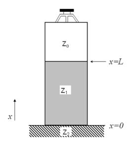
Fig. 1. Schematic of the impedance tube, partially filled with porous material.
