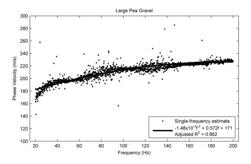
Fig. 4. Phase velocity for large sifted pea gravel.
