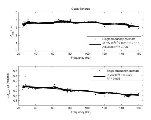
Fig. 8. Complex characteristic impedance of 10 mm glass spheres.
