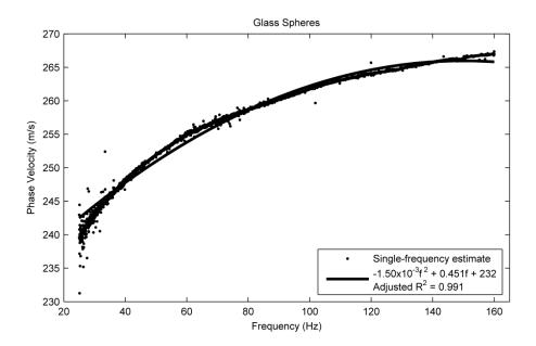
Fig. 7. Phase velocity of 10 mm glass spheres.
