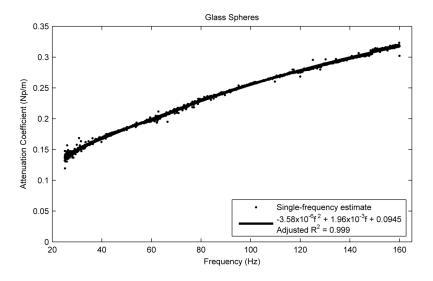
Fig. 6. Attenuation coefficient of 10 mm glass spheres.
