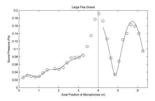
**Fig. 2.** Measured sound pressure amplitudes in large pea gravel at 100 Hz, with best fit function. Only 15 of the pressures in the gravel and 11 pressures in the air are fitted, owing to equipment limitations.
