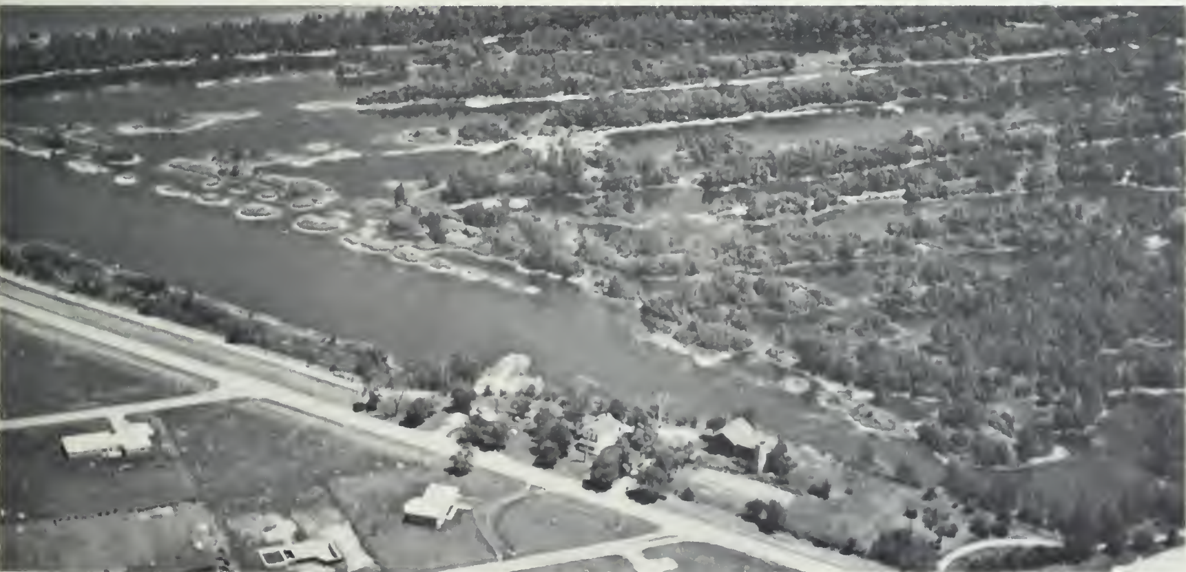
Fig. 21 – Lost Potential: A Water Area Choked with Overburden from an Unplanned Dragline Operation
