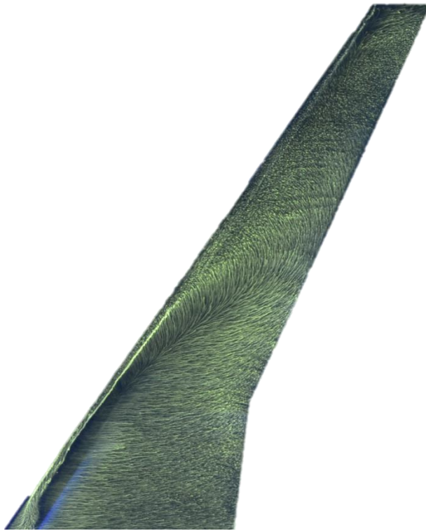
Fig. 4.3 Oil flow of the stalled clean wing, \alpha = 9.6^\circ , Re = 3 \times 10^5 .
