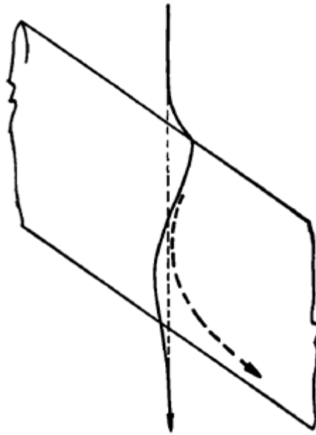
Fig. 2.5 Path of a particle outside of the boundary layer (full line) and inside the boundary layer (dashed line). 11
