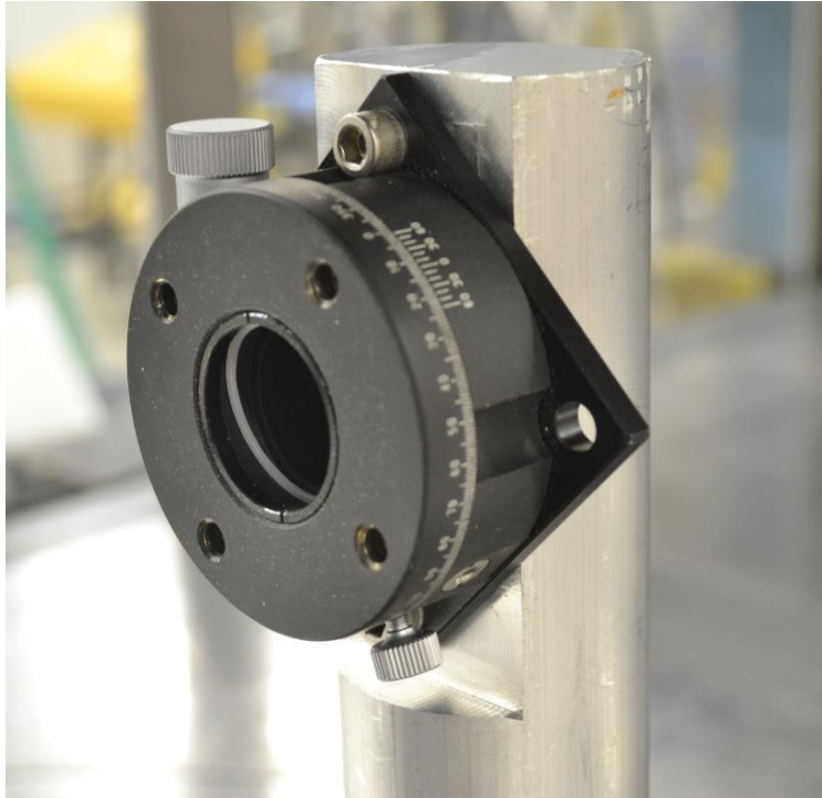
Fig. A.5 Manual rotation stage used to set the roll angle of the probe.
