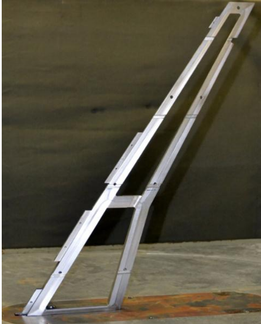
Fig. 3.3 Steel frame for wind tunnel model.
