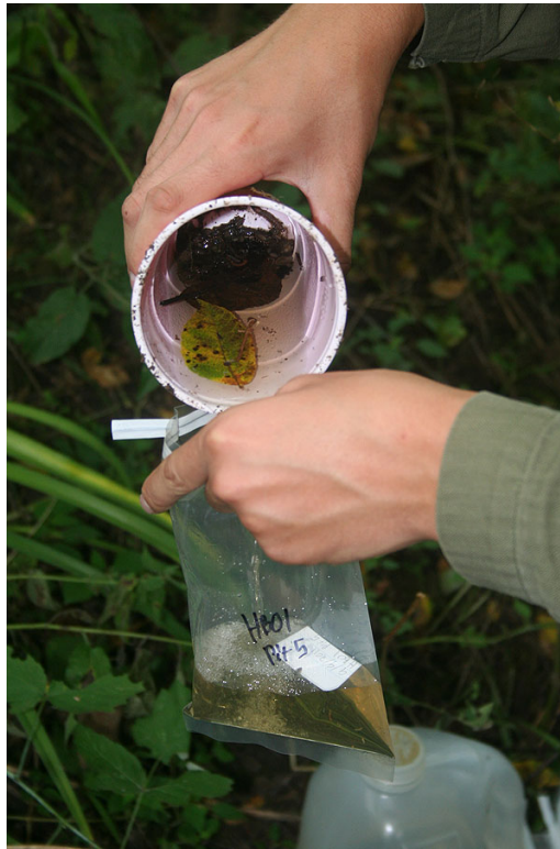
Figure 6. Pouring propylene glycol and sample contents into double-labeled sample bag at end of sampling period, Hanover Bluff 01, 9 September 2011.
