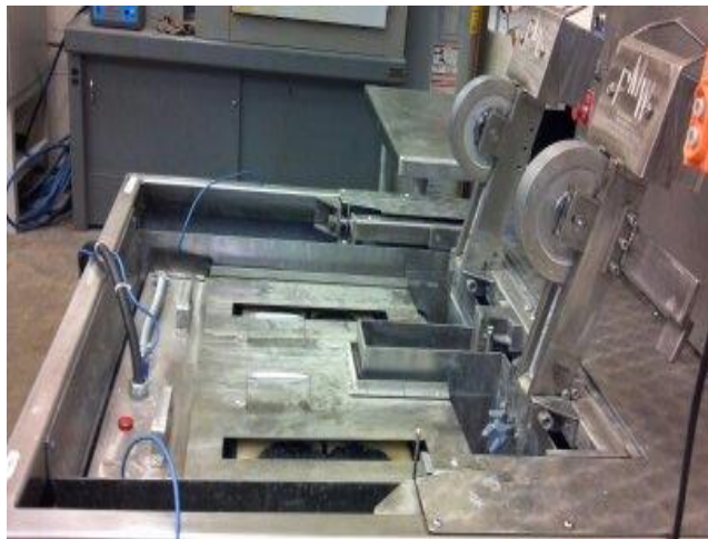
Figure 4.2. Hamburg loaded-wheel track test setup under dry and heated conditions.
