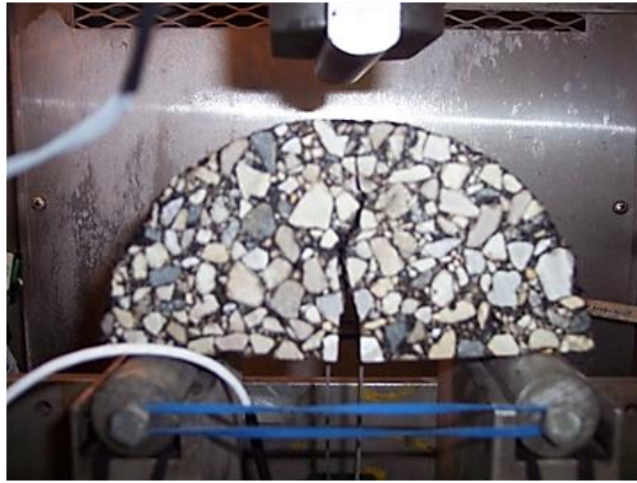
Figure 4.7. Failed SCB test specimen.
