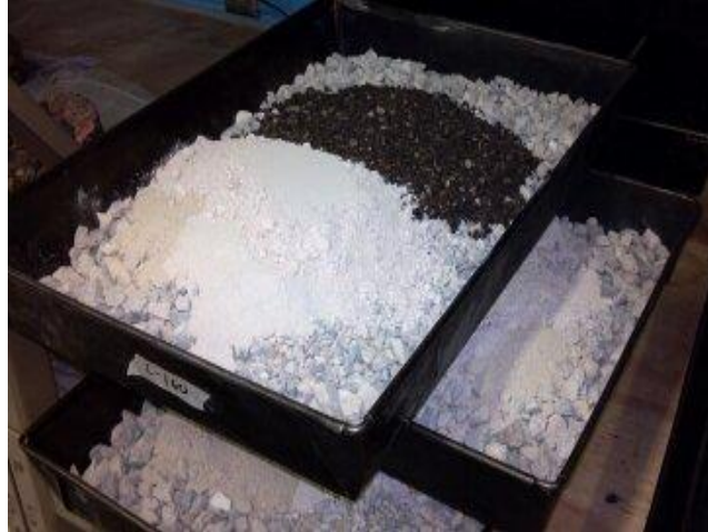
Figure 3.2. Batched SMA aggregates with FRAP and mineral filler.
