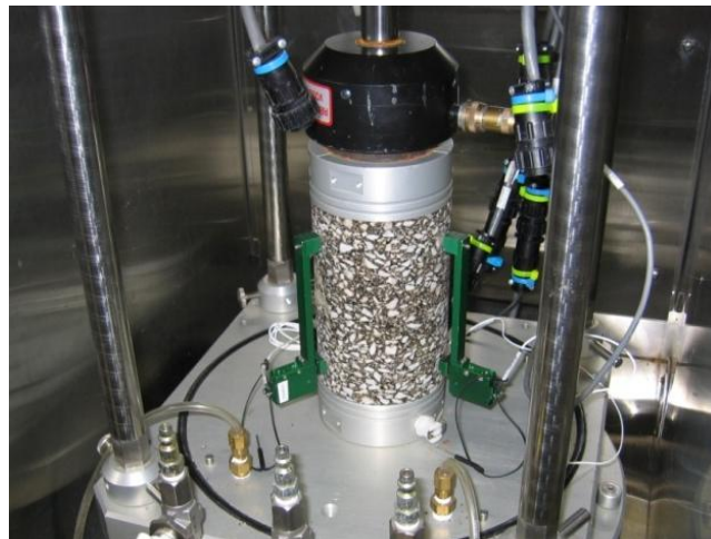
Figure 4.1. Complex modulus setup with extensometers attached onto the specimen.
