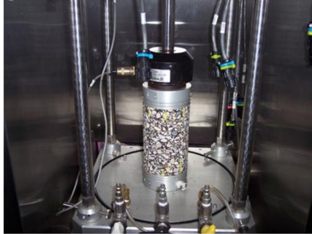
Figure 4.4. Flow number test setup.
