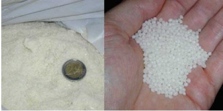
Figure 2.1. Sasobit flakes (left) and prills (right) (11).
