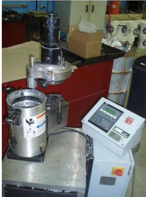
Figure 3.5. Portable gyratory compactor for specimen preparation.
