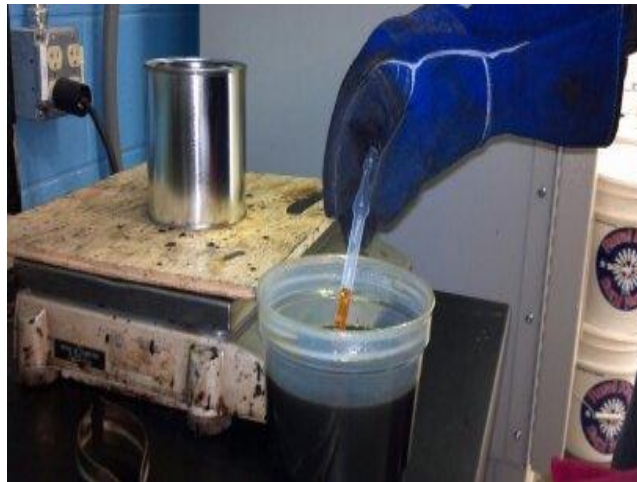
Figure 3.3. Addition of the chemical WMA additive to asphalt binder.
