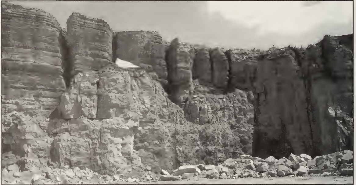
Figure 21 Highwall at Savanna Blacktop and Quarry; karst solution features can be seen in the Ordovician dolomite near the top (photo by W. T. Frankie).
