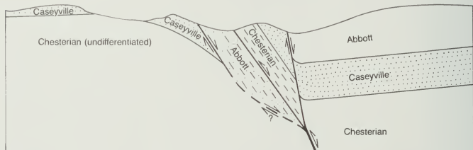
Figure 39 Profile of Lusk Creek Fault Zone in SW Section 35, T11S, R6E (see fig. 37 for line of section). The fault zone contains two slices. The southeastern slice, containing Chesterian and Caseyville strata, is upthrown relative to rocks on either side. The northwestern slice of Abbott Formation is downropped relative to rocks on both sides. Net displacement and final motion was normal, down to the southeast.
