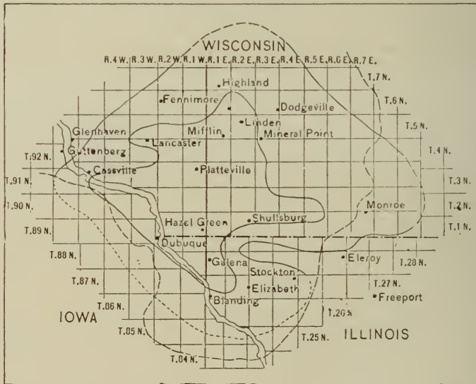
FIG. 2. Map showing distribution of the oil-rock. The outer continuous line marks the outer boundary of the area underlain by oil-rock. Where broken, boundary is uncertain. The inner continuous line incloses the area over which the oil-rock averages a foot or more in thickness. (This thickness includes only the pure oil-rock and not the interbedded clay and limestone which are often reported as oil-rock.) The line composed of dashes marks the edge of the non-glaciated district, from which the Maquoketa shale, except in a few small places, has been entirely eroded.
