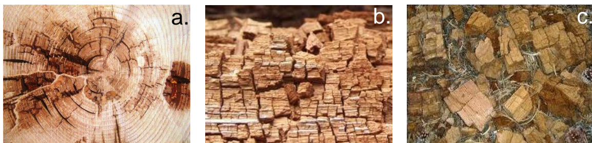
Figure 6. Examples of brown rot, a. brown rot in a timber cross-section, b. a log showing radial and tangential cracking, c. “cubes” of brown rotted wood.
