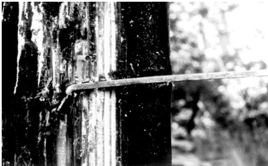
Figure 13. Shell-thickness indicator. The hooked end allows the inspector to identify rings and the edge of internal void. Figure extracted from Morrell [29].
