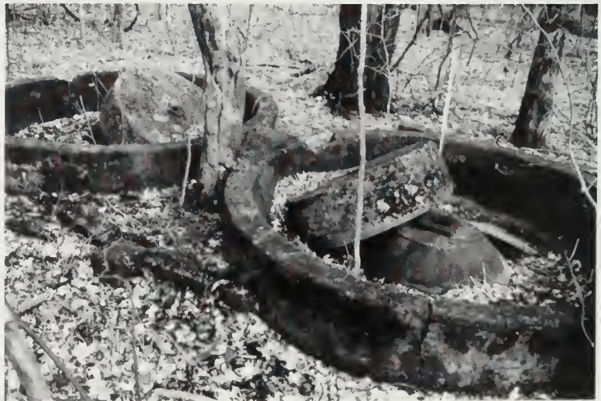
Figure 35 Twin "chaser" grinding mills of an abandoned silica plant in the SE, Sec. 33, T14S, R2W, Mill Creek Quadrangle. The limestone grinding wheels rolled around circular tracks to crush the silica.
