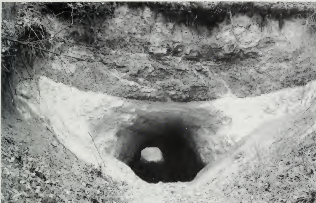
Figure 7 Abandoned underground silica mine in white tripoli of Clear Creek Formation, overlain by hard, fractured, brownish orange bedded chert. The tunnel was driven through the crest of a ridge; it served room-and-pillar workings within the ridge and also provided a haulage road to mines on the other side of the ridge. The location is in the SE NE, Sec. 23, T14S, R2W, Mill Creek Quadrangle.
