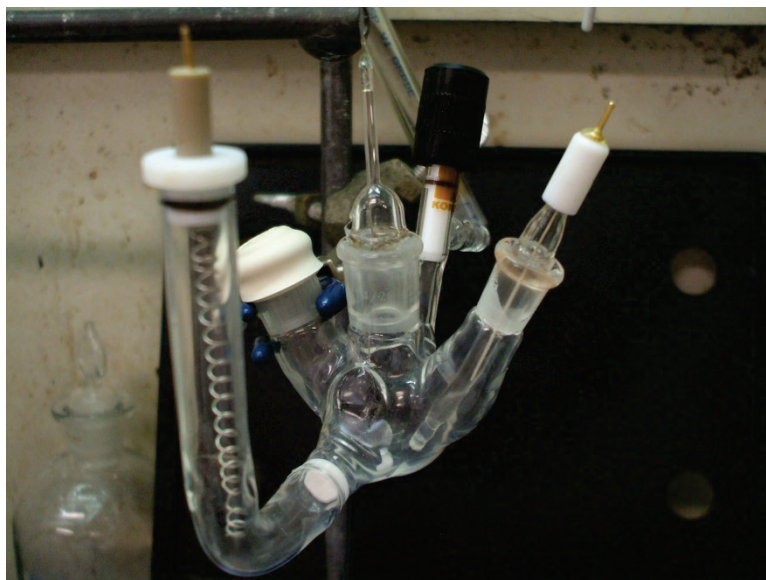
Figure 3.28. Controlled potential electrolysis cell, fitted with electrodes.
