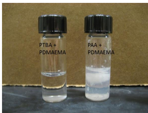
Figure 5.3 – Mixing of polymer solutions: PTBA and PDMAEMA in THF (left) resulting in no reaction, PDMAEMA and PAA in H 2 O (right) resulting in white precipitate.
