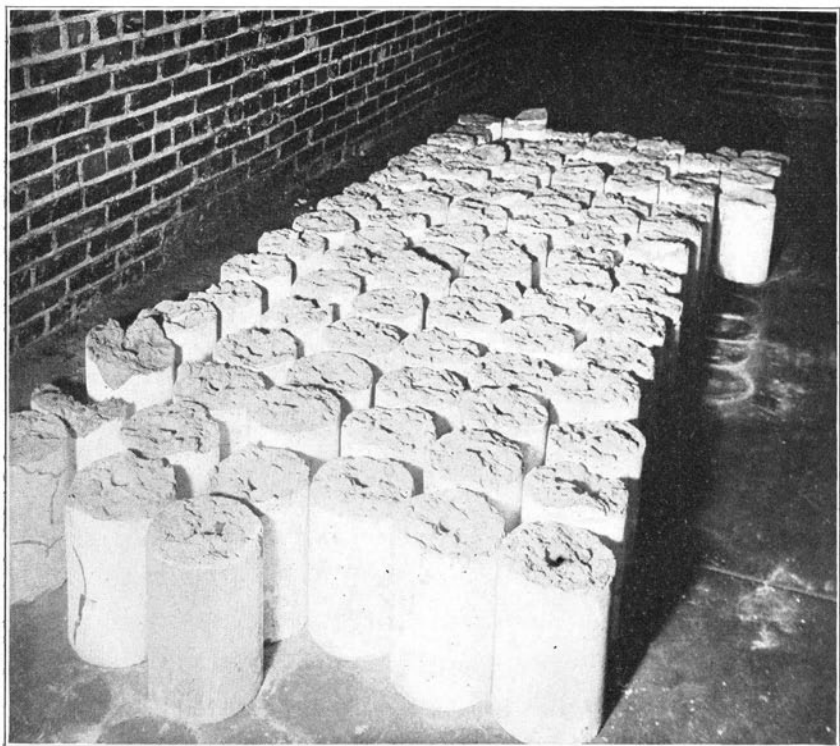
FIG. 6. GENERAL VIEW OF BROKEN TEST CYLINDERS
