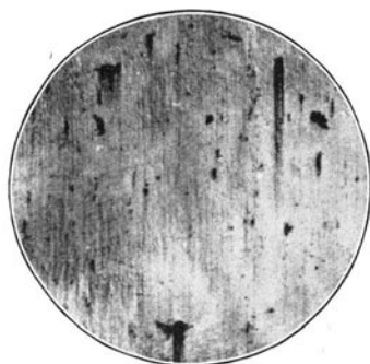
FIG. 41. MICROGRAPH OF SURFACE OF ROUGE-FINISHED SPECIMEN Magnification 100 diameters
