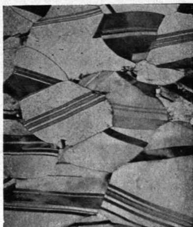
(a) 15 sec. at 500 deg. C. Recrystallization has just begun.
