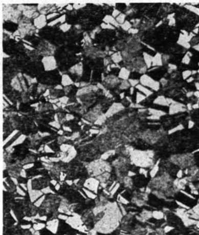
(d) 15 sec. at 650 deg. C. Av. G.S. = 0.027 mm. Considerable coalescence.
