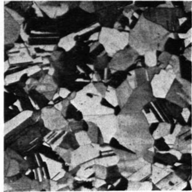
(f) 15 sec. at 650 deg. C. Av. G.S. = 0.086 mm.
