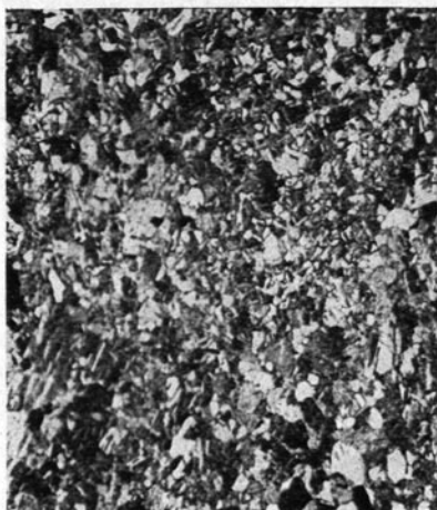
(a) 16 min. at 400 deg. C. Av. G.S. = 0.016 mm.
