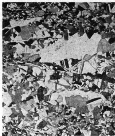
(c) 8 min. at 500 deg. C. Recrystallization almost complete.
