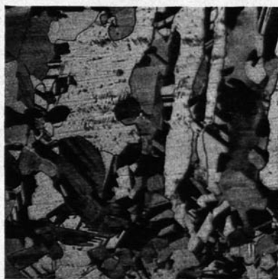
(a) 2 hr. at 450 deg. C. Not completely recrystallized.
