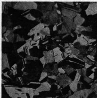
(b) 4 hr. at 450 deg. C. Av. G.S. = 0.093 mm.
