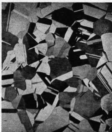
(f) 32 min. at 700 deg. C. Coalescence.
