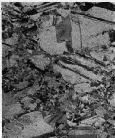
(b) 4 hr. at 400 deg. C. Partial recrystallization.
