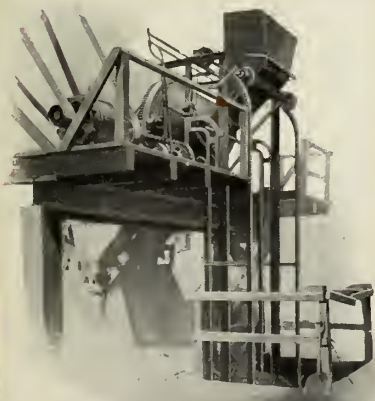
Figure 12—Smith Mixer with power-charging attachment, guide tracks extended
