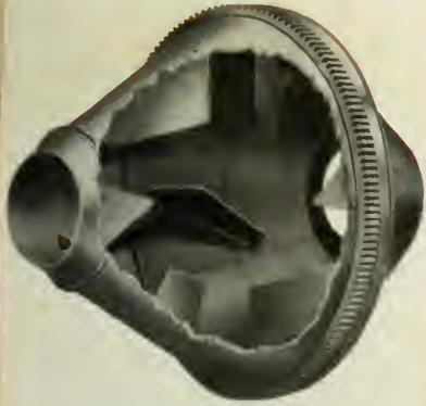
Figure 6—Sectional View of Smith Mixer Drum
